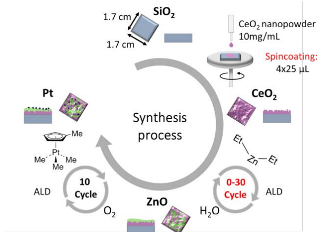
Figure 1. Synthesis procedure for the 10cPt_0-30cZnO_CeO 2 samples.
