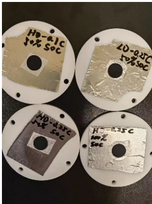
Fig.1. Lithium battery electrode samples in NDP chambers
