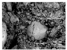
(c) With 20% CH. Fig. 1 Micrographs of AAM samples
