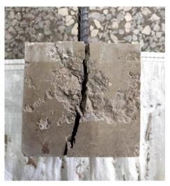
Figure 2 High-temperature spall of concrete.
