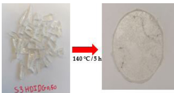
Figure 2. Recycling of S3HDI 0.5 DG 0.5 at 140 °C within 5 hours under a pressure of 10 MPa.
