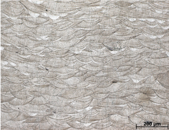
Fig. 2. Etched cross-section of the as-fabricated SLM maraging steel observed by OM
