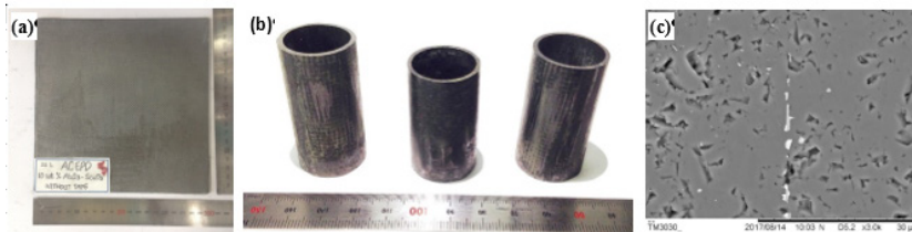
Fig 1. Images of the SiC f /SiC having (a) planar 200×200×3 mm 3 , (b) tubular with 20mm diameter and 50 mm height fabricated by EPD combined with hot pressing, and (c) the joining SiC f /SiC interface using Ti 3 SiC 2 filler, showing the possible elimination of the joining filler by solid-state diffusion.
